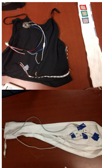
Figure 3: The top image shows the back of the vest along with the detachable cloth with patches. The bottom image shows the inside of the cloth with the patches connected with alligator clips
