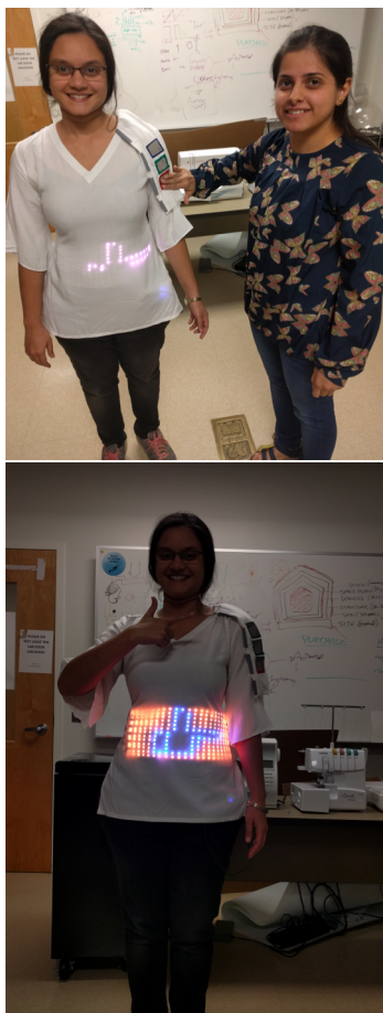
Figure 4: LEDs light up in different colors based on the touches. The image below shows the pattern that is revealed when 49 LEDs light up
