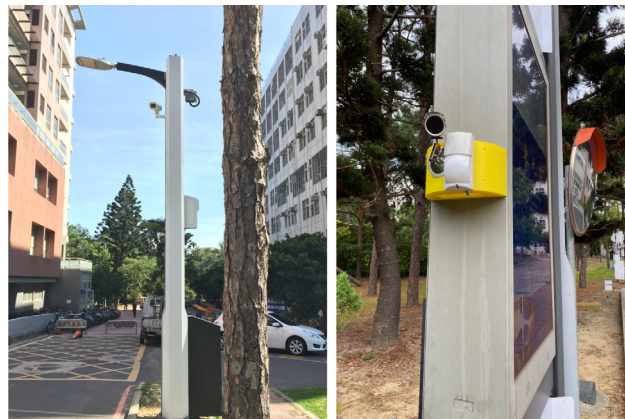
Fig. 9. Our testbed at NTHU campus, Taiwan: a smart street lamp (left) and a motion sensor (right).
